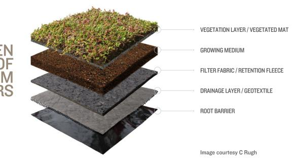
is because as the column height (= media depth) increases, the force of gravity on the water column, also called hydraulic head, leads to greater water loss at the upper levels of the media profile beginning immediately after a storm. In other words, the deeper the media profile, the drier the uppermost levels will be.
