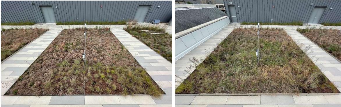
Figure 9. Visible plant stress during an extended dry period was greater in the 10 cm bed (left) than the 20 cm bed (right) following cessation of irrigation between January 2022 and July 20, 2022, on the APD-EGR. These two 5 September 2022 photos were taken by Lee R. Skabelund.
