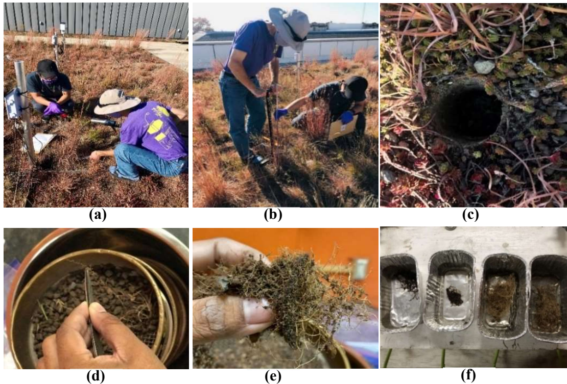
Figure 6. Collecting and analyzing root biomass samples from 10 cm and 20 cm deep APD-EGR beds. Photographs taken by M. M. Lekhon Alam, November 2020. (a) measuring consistent distance (~3–6 cm) from a plant; (b) trying to reach the bottom of the plot with a soil probe while also taking the height to determine h value for the analysis; (c) a volumetric core of soil was taken from the plot; (d) Large roots were hand-picked from the soil; (e) a portion of root biomass from a soil core; (f) Roots were gathered in a separate metal tin for each sample/plot.
